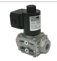
Open/close time less than 1 sec Max 16 operations per minute Media temperature -10 to 60 deg C Max inlet pressure 200mbar Aluminium body with female Rp threads 230VAC coil (110VAC and 24VAC option)
