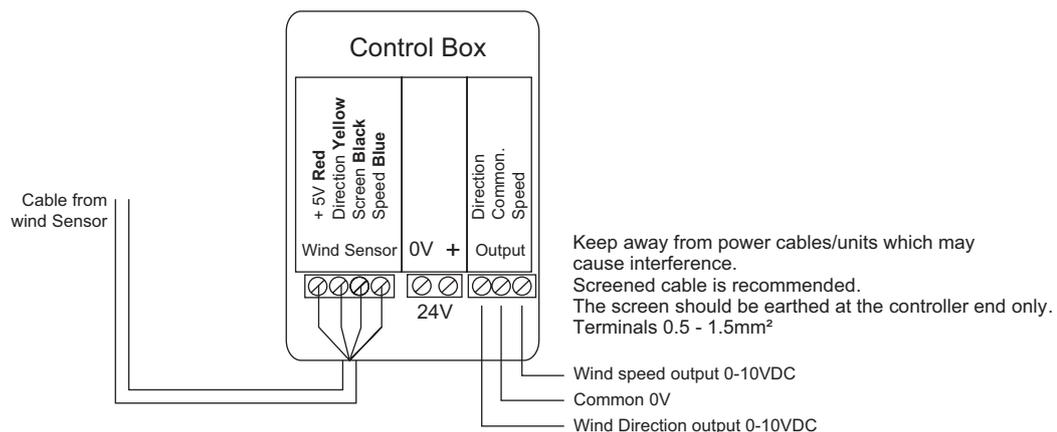
Supplied with the control box which converts the sensor signal to a standard 0-10 volt output signal.
