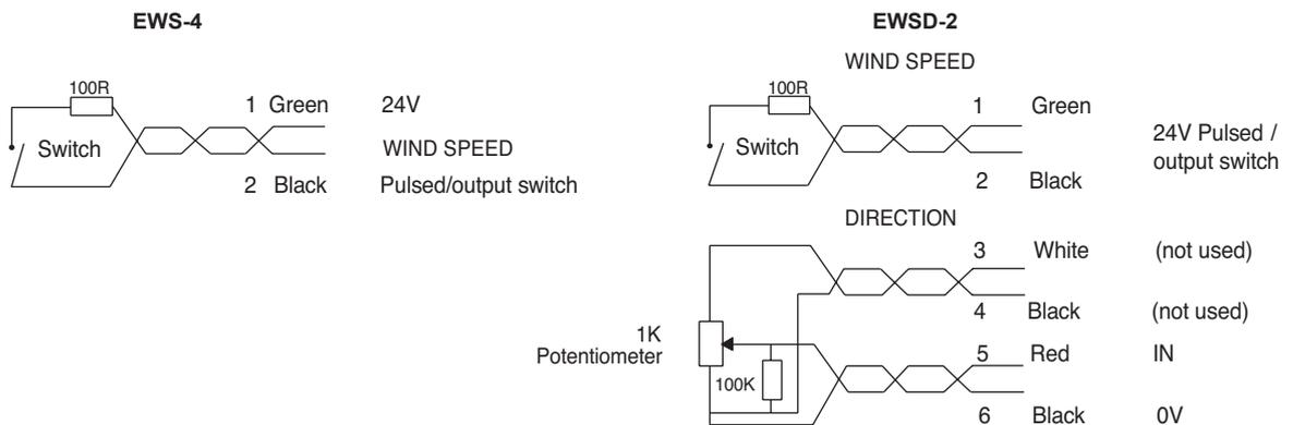
The 3m cable can be extended using screened 7/0.2mm wire equivalent to Belden 9503. The screen is not connected in the sensor and should be earthed at the controller end. Keep away from power cables/units which may cause interference.
