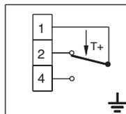
Open low = Contact 1 - 4 opens on temperature fall.. Temperature must rise to allow resetting
